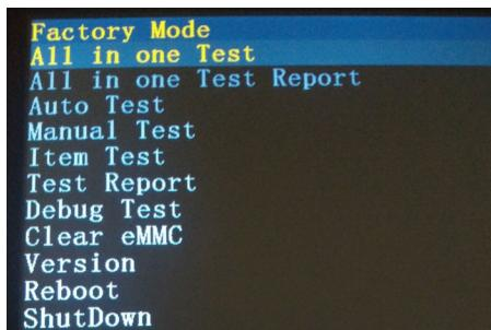
You can access this menu by pressing and holding the volume down button. (Factory Mode)
